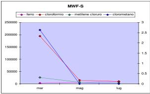
**Summary:** During the four month demonstration at a pharmaceutical manufacturing site near Milan, Italy a single ART system reduced chloroform and methelyene chloride concentrations in groundwater by more than 98%. As a result of monitoring contaminant concentrations in groundwater it was determined the radius of influence of the ART system was greater than 9 meters.
